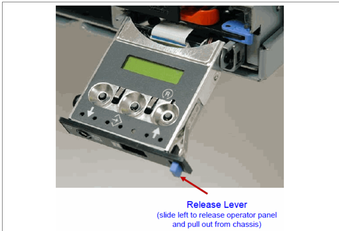
Figure 4-7 Operator panel is pulled out from the chassis
