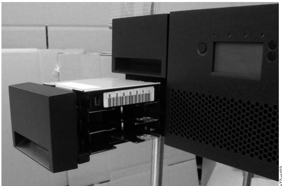
Figure 2-36. 4U library I/O Station in the lower left magazine
