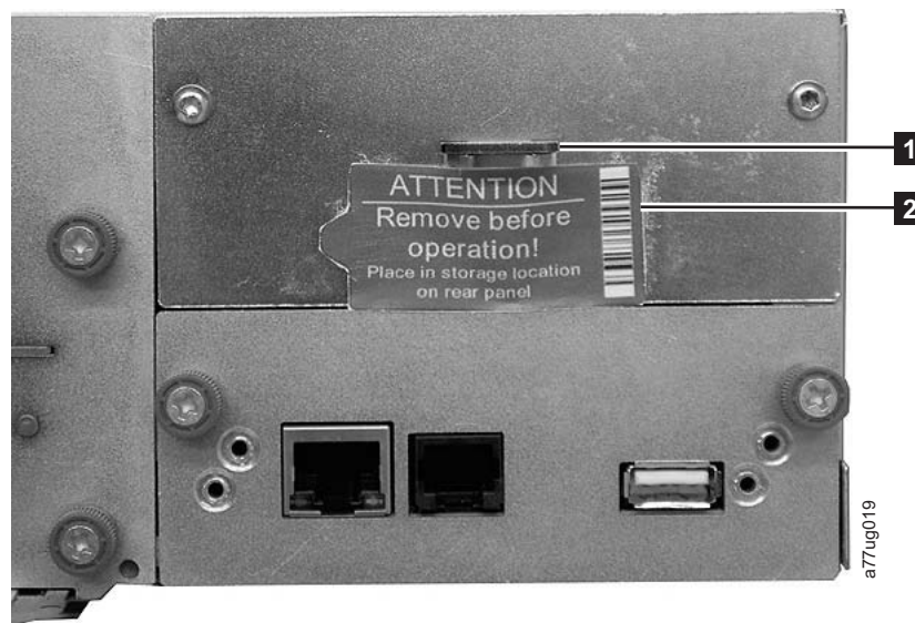
Figure 2-3. Library shipping lock and label storage location
